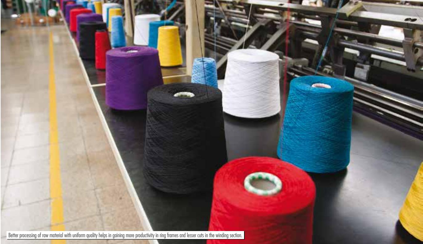
Better processing of raw material with uniform quality helps in gaining more productivity in ring frames and lesser cuts in the winding section.
